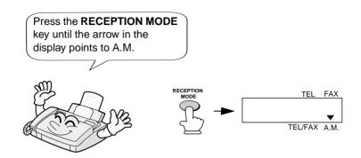
In A.M. mode, your fax will automatically receive voice and fax messages if you have connected an answering machine to the fax machine. See Chapter 6 for more details.
